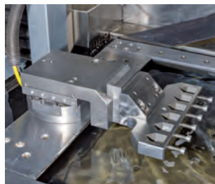
Smart-Grip AIR with adjustment pallet 3D and 6-fold prism
