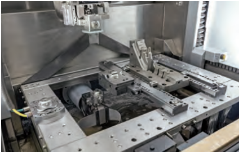
Smart-Grip BAR Vice-Slide and Slide as well as pallet carrier Smart-Grip AIR
