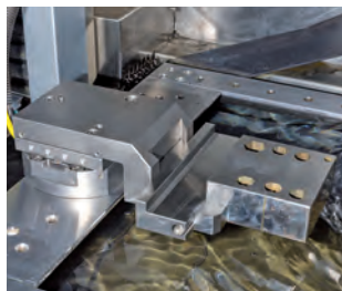
Smart-Grip AIR with adjustment pallet 3D and Smart vice 0 – 120 mm
