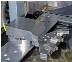
Smart-Grip AIR with pallet fix and Flange system 3R ICS
