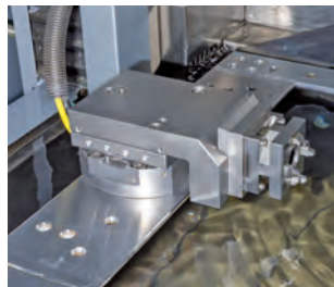
Smart-Grip AIR with adjustment pallet 3D and EROWA Quick Chuck 50
