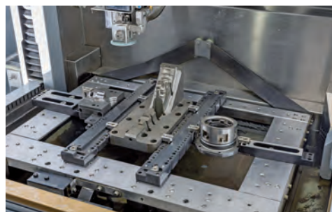
Smart-Grip BAR Vice-Slide and Slide as well as clamping jaw double and simple
